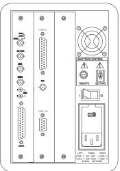
Figure 1. Power Switch Location (ST-133A and ST-133B)
